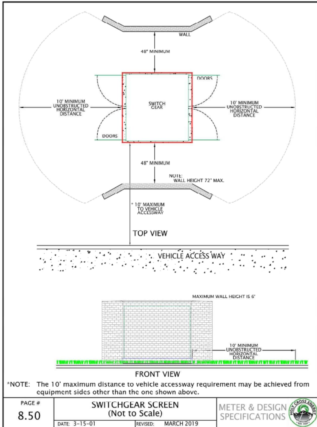
\*NOTE: The 10' maximum distance to vehicle accessway requirement may be achieved from equipment sides other than the one shown above.
