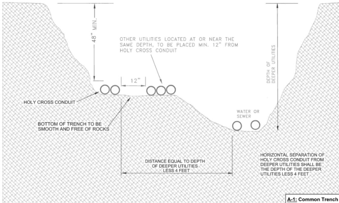
9. Power line conduits will be installed with a minimum separation of 12" from all other new or existing underground utility lines. Wherever possible, this separation will be horizontal. The 12" of separation shall be maintained when crossing other utilities in the trench. Whenever possible, gas line crossings should have 3' of separation from HCE conduit.
